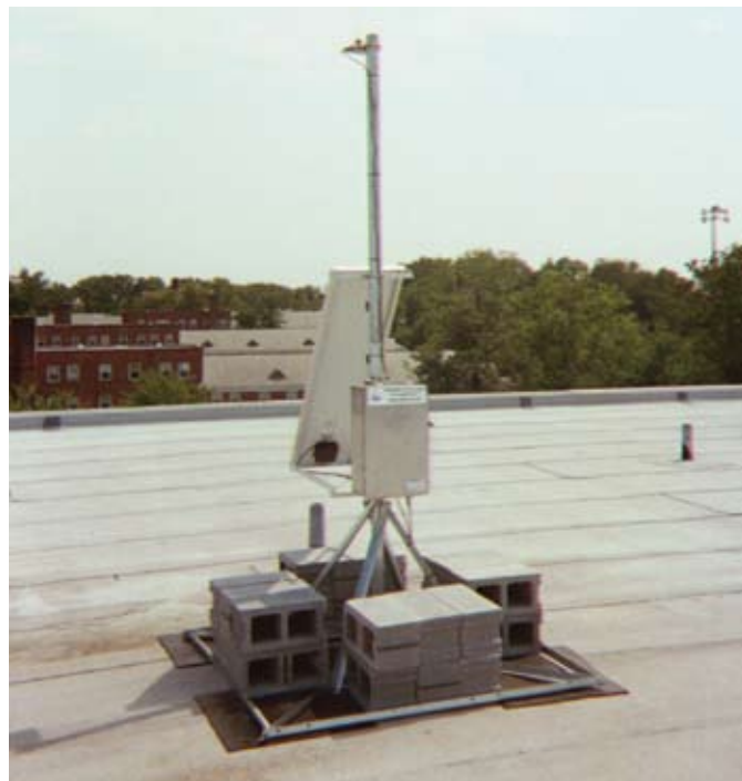
Data collectors for the STAR Network system are located on light poles and building roofs.
